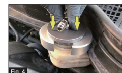
4.Press the adapter down into the master cylinder reservoir filler neck.
