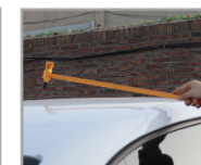
4. Can use assembled logn hammers to strike distant dents.
