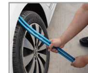
3. Using the wheel hub as a support, press and repair the dents that need to be repaired.
