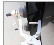
3. Install the applicable repair head and align it with the unevenness that needs to be repaired.
