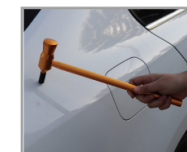
3. Short hammers can be used to repair dents.
