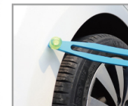
4. For different dents, a decoration compound can also be installed at the top of the sliding rod for repair.
