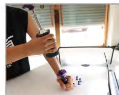
3. Pull the slide hammer hard to perform lifting repair.
