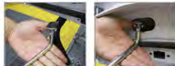
1. As shown in the picture, install the top head on the crowbar.
