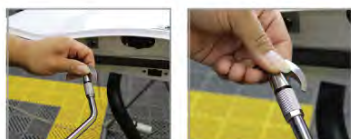
1. The swivel head is mounted on the crowbar. 2. Rotate the top to the appropriate position.
