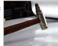
1. The big head can be used to knock and repair large bumps.
