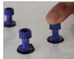
1. Use the pull tab to stick to the dent.
