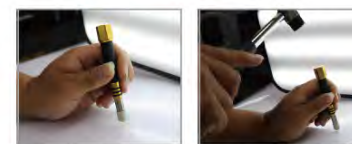
1. Align the area that needs repair. 2. Use a hammer to repeatedly tap the top of the repair pen.
