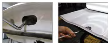
3. Reach under the indentation inside the car body. 4. Restoration work with movable crowbar.
