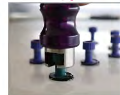
2. Install the pull tab on the groove of the slide hammer
