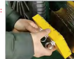
1. Glue the pull strip with hot melt adhesive to the concave area.
