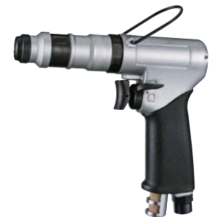
■ ARW-9486 1/4" HEX. SUPER DUTY FULL-AUTO SHUT OFF AIR SCREWDRIVER -1,700RPM · Handle Exhaust With Muffler
