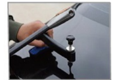
2. Align the repair pen with the protrusion, and trim it with the beat.
